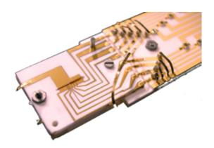
This image shows the ion trap used in the experiment. Electrical potential are applied through thin gold wires on a chip and used to trap ions in a narrow slot. Credit: NIST
