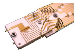
This image shows the ion trap used in the experiment. Electrical potential are applied through thin gold wires on a chip and used to trap ions in a narrow slot. Credit: NIST
