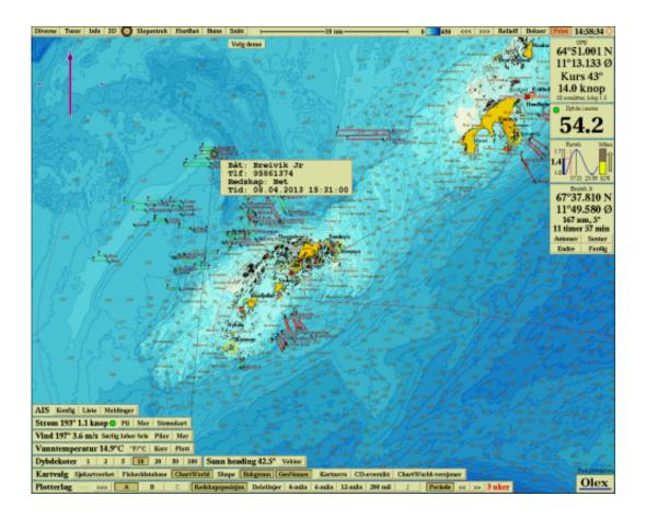
Map plotter display of the area offshore Røst in April 2013. Red lines show the locations of autolines. Nets are shown in green and the red dots are crab pots. By moving the pointer to the beginning of a line, the vessel's number and type of equipment can be displayed.
