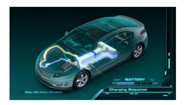
The 2011 Chevrolet Volt's 16 kWh battery can be recharged using a 120V or 240V outlet. The car's lithium-ion battery is based on technology developed at Argonne. Credit: General Motors.
