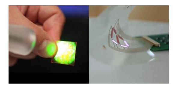
The prototype laser detection device, which can be used to protect goods against counterfeiting. Right: Printed electronics enable flexible, digital displays which can be bent without breaking. Credit: Nick Saffell
