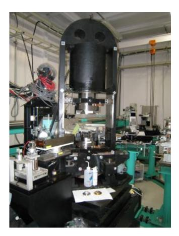
The high pressure apparatus installed on the beamline BL14B1 at SPring-8, a third generation synchrotron radiation facility in Japan. Credit: H. Saitoh/JAEA
