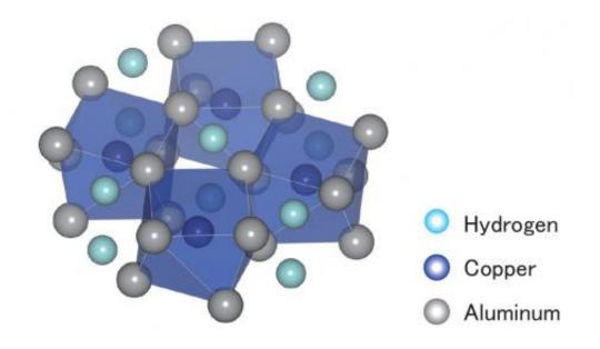
This is a schematic of the hydrogenation reaction process of the newly developed hydride Al2CuHx. Credit: H. Saitoh /JAEA
