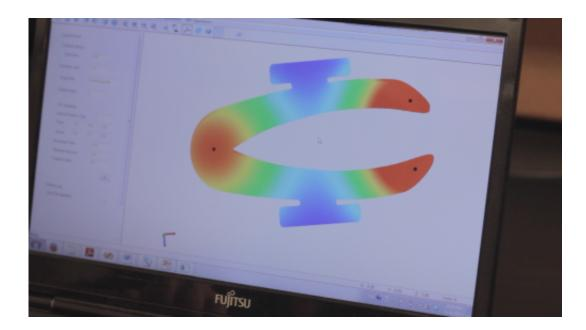
A computer model of a pair of tweezers shows the distribution of materials and degrees of hardness in the object to be 3D-printed in Dr. Yong Chen's lab at USC Viterbi. Credit: USC Viterbi
