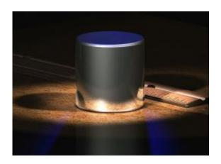
A computer-generated image of the International Prototype kilogram (IPK), which is made from an alloy of 90% platinum and 10% iridium (by weight) and machined into a right-circular cylinder (height = diameter) of 39.17 mm. The IPK is kept at the Bureau International des Poids et Mesures (International Bureau of Weights and Measures) in Sčvres on the outskirts of Paris.
