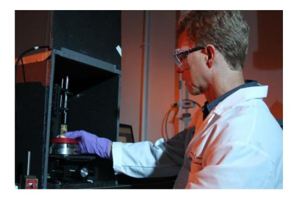
Greg Klunder, a chemist in LLNL's Forensic Science Center, examines a uranium ore concentrate sample with the aid of a near-infrared spectrometer. Credit: Steve Wampler/LLNL
