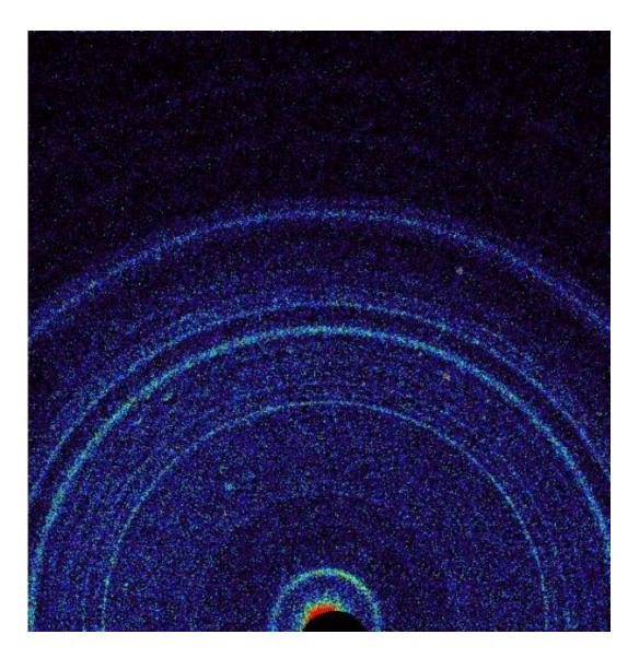
The x-ray diffraction pattern Curiosity sent down after analyzing scoop number 5. To a mineralogist, the concentric rings are like a fingerprint, revealing the structure and chemistry of a particular mineral. Credit: NASA/JPL-Caltech/Ames
