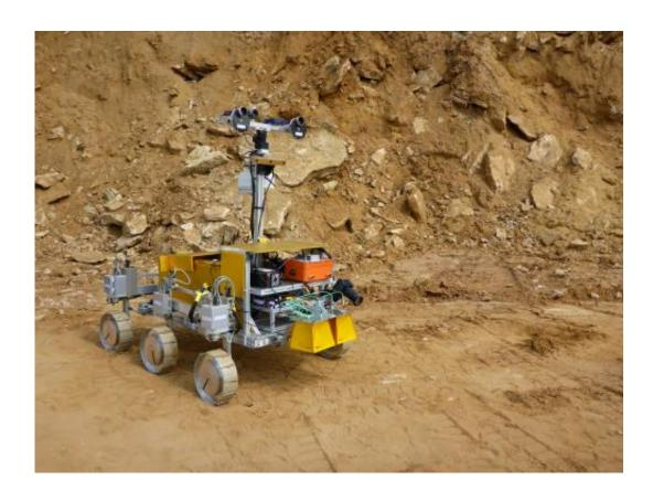
An early ground prototype of ESA's six-wheeled ExoMars rover vehicle, nicknamed 'Bridget', was used for the SAFER (Sample Acquisition Field Experiment with a Rover) field test in Chile's Atacama desert during October 2013. This photo was taken during a preliminary run in Upwood Quarry near Abingdon in Oxfordshire, UK, in July 2013. Credit: ESA-Michel van Winnendael
