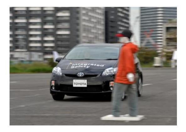
Toyota Motor demonstrates its "pre-collision system", which uses automatic steering in addition to automatic braking to prevent collisions, in Tokyo, October 10, 2013
