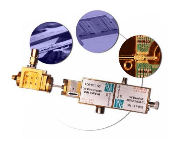
The dimensions of the receiver are approximately 17 cm x 3 cm. From left, the three circles show: 1. A SEM image of a 557-GHz Schottky mixer membrane circuit. 2. A SEM image of a 278-GHz HBV tripler circuit. 3. A photograph of a 93-GHz mHEMT MMIC x6 multiplier module. Credit: Chalmers, IAF, Wasa Millimeter Wave
