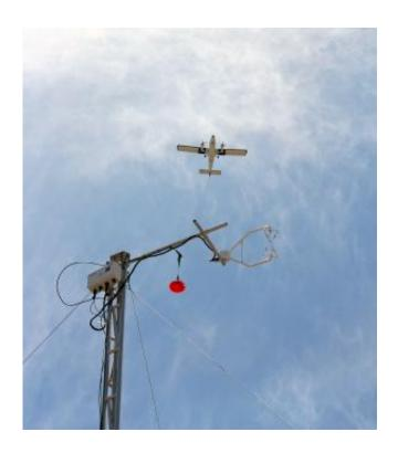
Aircraft overflight of the methane and meteorological sensing towers deployed by Los Alamos National Laboratory at the South methane controlled release site. Credit: JPL/Los Alamos
