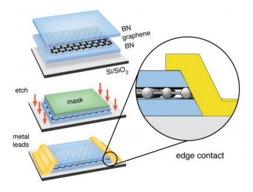
This is an illustration of an encapsulated two-dimensional graphene sheet that is electrically contacted only along its one-dimensional edge. Credit: Columbia Engineering; Illustration, James Hedberg and Cory Dean
