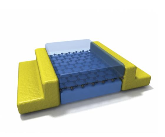
After first encapsulating graphene in boron nitride, the multilayer stack is etched to expose only the very edge of the two-dimensional graphene layer. Electrical contact is then made by metalizing along this one-dimensional edge. Credit: Columbia Engineering; illustration, Cory Dean
