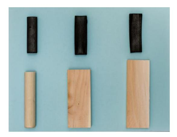
Any kind of wood can be made into biochar by heating in a low-oxygen chamber. Some types of wood work better than others. Pictured (left to right) are white birch, white pine and red cedar. Credit: L. Brian Stauffer
