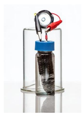
This corncob-biochar supercapacitor generates enough energy to power an LED bulb. Wood biochar is easier to use in large-scale applications and has more energy potential. Credit: L. Brian Stauffer
