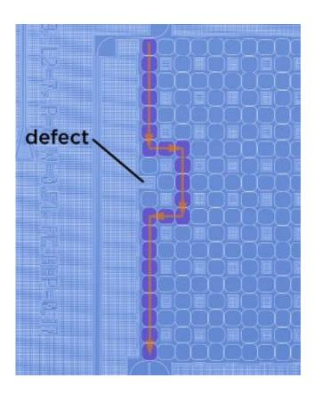
In this false-color scanning electron microscope image, the arrow shows the path light takes as it hops between silicon rings along the edge of the chip, successfully avoiding defects -- in this case a missing ring. Credit: NIST
