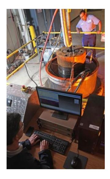
SwRI has added five, 13-inch-diameter chambers in its Ocean Simulation Laboratory for deep water simulation testing. The chambers are capable of attaining pressures of 30,000 psig at a rated temperature of 650 degrees F.
