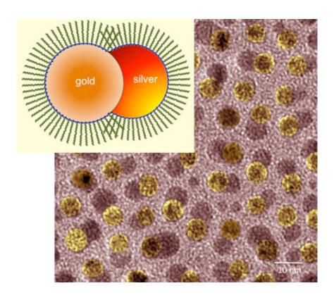
Silver and gold nanoparticle heterodimers (about 10 nm across); green wavy lines represent surfactant molecules in the schematic. Underlying is a TEM image of gold (golden color) and silver (dark gray) nanoparticles after epitaxial overgrowth for 180 sec.
