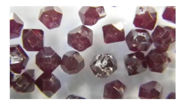
Microscope picture of small diamonds, 100 microns in diameter. Specific lattice defects do not only impart colour on the diamonds but also provide the basis for the magnetic field sensor. In their experiments the team at Ulm ground down these diamonds to a size of 20 nanometers (as a comparison, a human hair has a diameter of 70 microns and is therefore 3000 times thicker than the nanodiamonds). Credit: Fedor Jelezko
