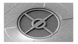
The silicon ring is a fast and effective switch for a beam of light skimming close to its edge. Credit: 2013 A\*STAR Institute of Microelectronics
