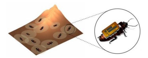
Researchers from North Carolina State University have developed software that allows them to map unknown environments -- such as collapsed buildings -- based on the movement of a swarm of insect cyborgs, or "biobots." Credit: Edgar Lobaton
