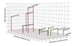
Rice University researchers have created a chemical sensor to identify solvent fumes by their fluorescent "fingerprints." Three unique characteristics for each type of vapor — the average lifetime, intensity increase and emission maxima — allowed the researchers to plot them on a 3-D map. Credit: Angel Martí/Rice University
