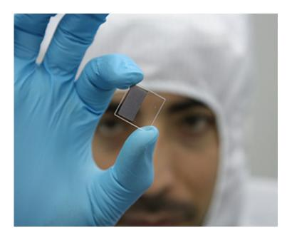
PhD student Ali Sardarinejad holding a thin film of ruthenium oxide used in the new pH sensor.
