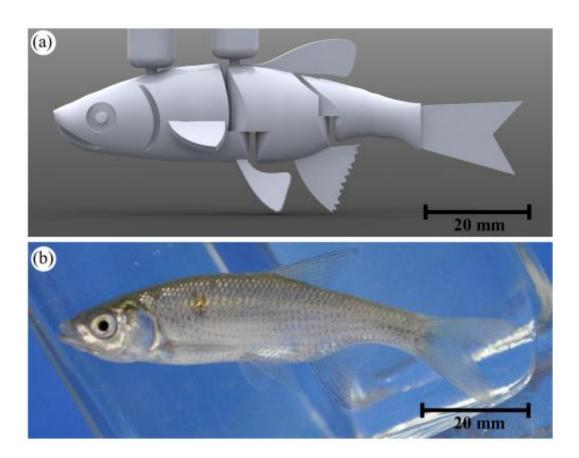
Researchers at NYU-Poly designed a bio-inspired robotic fish that imitates a golden shiner. Experiments revealed the live fish would swim closer to the robot that was painted with a more natural palette, particularly when the robot mimicked the tail beat of a real fish. Credit: *PLOS ONE*
