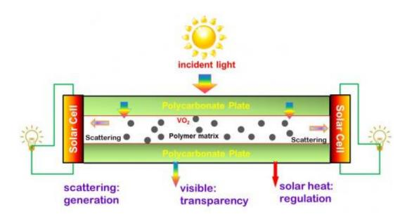
A hybrid smart window device that can achieve energy savings and generation was designed based on a sandwiched composite film that was composed of dispersed VO2 particles and a polymer matrix. This device can temperature-dependently regulate solar heat and generate electricity using a solar cell positioned around the glass panel and powered by VO2 particle-scattered light, simultaneously remaining visible transparency. Credit: J. Zhou, Z. Chen and Y.F. Gao
