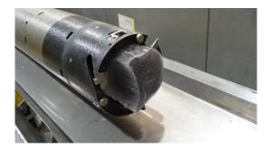
This chunk of ice has made history. A National Science Foundation-funded Replicate Core Drilling Team was able to retrieve cylinders of ice from the original ice core hole while leaving the borehole intact.
