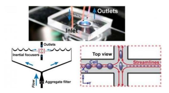
This is the experimental setup for imaging flow cytometry. Credit: Jacobs School of Engineering/UC San Diego
