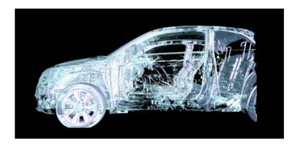
Through the eye of the XXL CT scanner: A car reveals its innermost secrets at the Fraunhofer Development Center for X-ray Technology EZRT in Fürth. Credit: © Fraunhofer IIS
