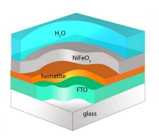
Taking Mother Nature's lead, researchers have sought new methods and materials capable of mimicking photosynthesis. Researchers at Boston College report that modifying the surface of hematite with a nickel iron oxide coating produces an increase in cathode photovoltage of nearly four-tenths of a volt. That's nearly enough energy to put an economical method of artificial photosynthesis within reach. Credit: *Angewandte Chemie*
