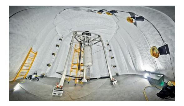
The Large Underground Xenon experiment installed 4,850 ft underground inside a 70,000 gallon water tank shield. The experiment is a 370 kg liquid xenon time projection chamber that aims to detect the faint interactions between WIMP dark matter and ordinary matter.
