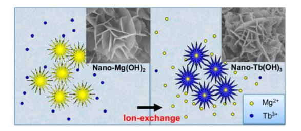
Many of today's technologies, from hybrid car batteries to flat-screen televisions, rely on materials known as rare earth elements (REEs) that are in short supply, but scientists are reporting development of a new method to recycle them from wastewater. The process, which is described in a study in the journal *ACS Applied Materials & Interfaces*, could help alleviate economic and environmental pressures facing the REE industry.
