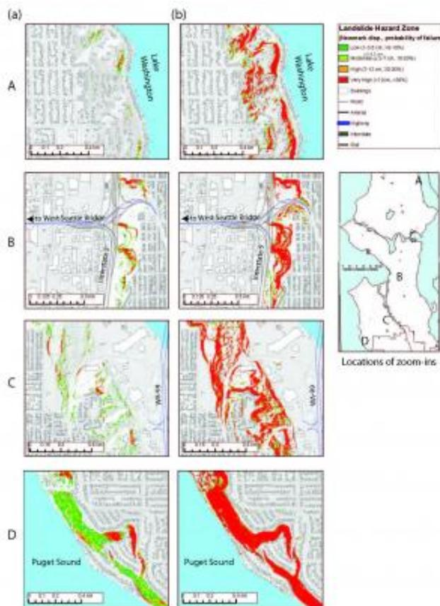
Locations of each zoom-in are shown on the map of Seattle at right. A) Coastal bluffs in the northern part of Seattle are most affected when soils are saturated. B) There are several areas along the I-5 corridor that are highly susceptible to landsliding for all soil saturation levels, such as the area shown here near the access point to the West Seattle bridge. C) The hillsides in West Seattle along the Duwamish valley are at risk of seismically induced landsliding, such as the area
