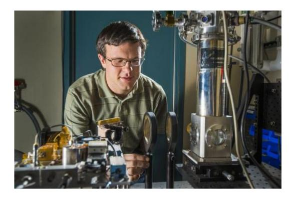
Sandia National Laboratories researcher Greg Dyer aligns a plasma-containing crystal that is tunable by varying the voltage. The technology potentially could increase the bandwidth of high-speed communications networks. Credit: Randy Montoya, Sandia National Laboratories
