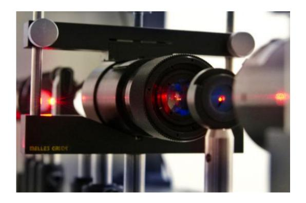
A demonstration set-up in Mohsen Kavehrad's lab creates partially coherent visible (red) light. This type of light performs better through the atmosphere than pure coherent light, an important consideration for outdoor optical wireless applications. Credit: Patrick Mansell
