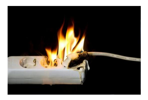
Many multi-plug connectors pose a fire risk, as they can overheat if the current flow is high. Flame retardants in the connector can prevent fires or slow the spread of the blaze. Credit: © Fraunhofer LBF
