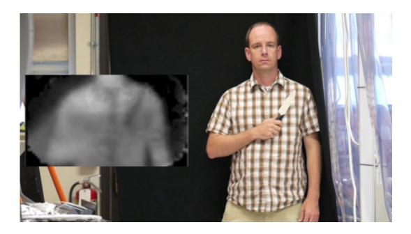
Researcher Dan Becker demonstrates NIST's prototype imaging system for remote detection of hidden weapons. The inset on the left is the image created by the instrument, which detects naturally emitted or reflected light at submillimeter wavelengths. The ceramic knife is cooler and reflects cooler light from the room, and therefore appears darker than the surrounding image. Credit: Becker/NIST
