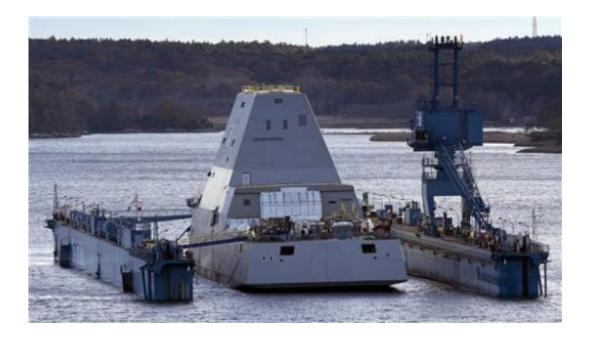
The first-in-class Zumwalt, the largest U.S. Navy destroyer ever built, floats off a submerged dry dock in the Kennebec River, Monday, Oct. 28, 2013, in Bath, Maine. Unlike warships with towering radar- and antenna-laden superstructures, the Zumwalt will ride low to the water to minimize its radar signature, making it stealthier than others. (AP Photo/Robert F. Bukaty)
