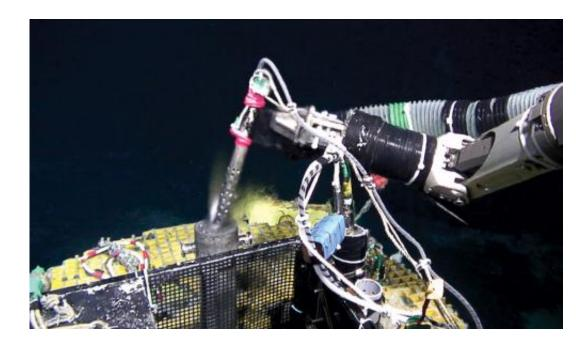
The robotic system inserts an electrode into hydrothermal fluid released from deep-sea vents in order to generate electricity. enlarge image Credit: © 2013 WILEY-VCH Verlag GmbH & Co. KGaA, Weinheim
