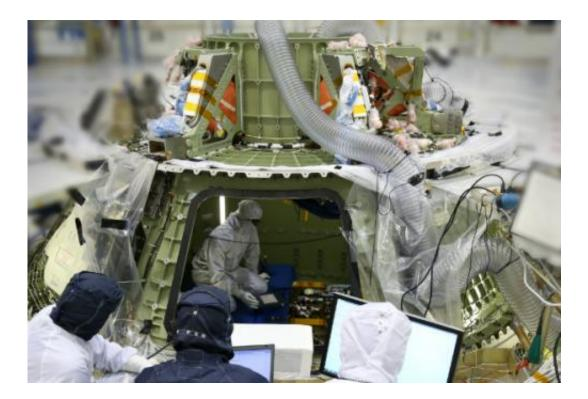
Orion's avionics system was installed on the crew module and powered up for a series of systems tests at NASA's Kennedy Space Center in Florida last week. Credit: Lockheed Martin.
