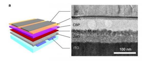
The quantum dot device structure shown with a transmission electron microscopy (TEM) image of a cross-section of a real device. Credit: Los Alamos National Laboratory
