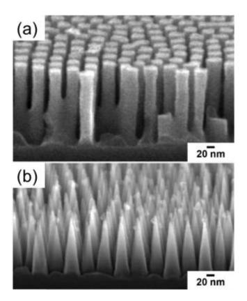
This is a side view scanning electron microscope image of a silicon surface textured with (a) cylindrical pillars and (b) nanocones. Credit: Brookhaven National Laboratory
