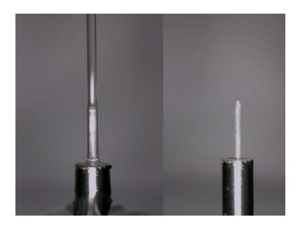
Shown is a close-up of the liquid jet sensor with the liquid jet (left) and without it (right). The jet of water is less than a millimeter in diameter. Credit: Gianluca Persichetti, IREA &#8211 CNR
