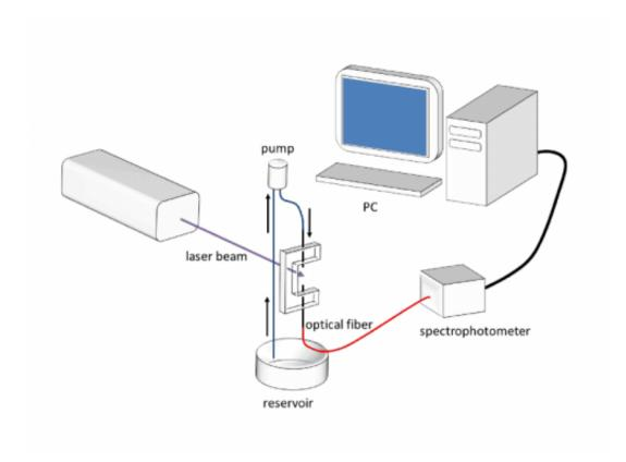
This is a schematic illustration of the technique used to detect contaminants. A laser beam is directed perpendicularly into the flow of water. Fluorescent light from contaminants in the water is carried away to be detected and analyzed. Credit: Gianluca Persichetti, IREA &#8211 CNR
