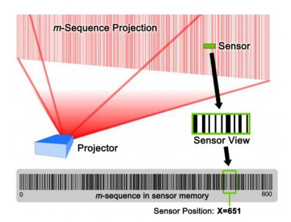
Lumitrack enables high-speed, high-precision tracking by projecting a barcodelike pattern, or m-sequence, over an area. A sensor can determine its position based on the unique portion of the m-sequence pattern it can detect. Credit: Carnegie Mellon University
