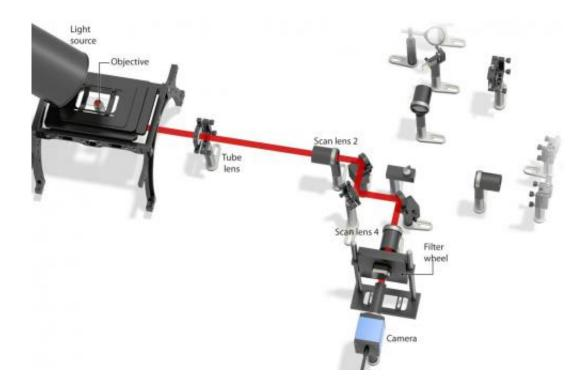
A lamp is used to illuminate the sample from above. Transmitted light is collected via the objective, passed through the Tube lens and Scan lens 2, and directed through Scan lens 4 via removable mirrors before imaging onto the camera. Credit: NIBIB
