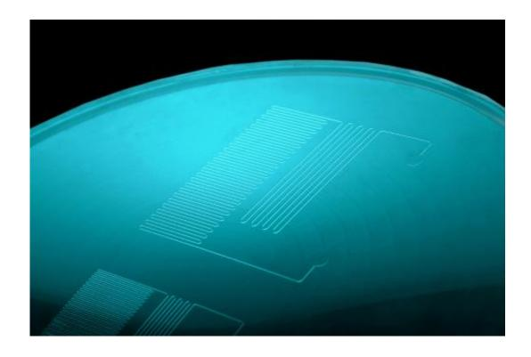
Microfluidic negative for structuring films. Credit: © Fraunhofer IPT
