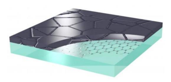
Graphene was deposited onto a glass substrate. The ultrathin layer is but one atomic layer thick (0.3 Angström, or 0.03 nanometers), although charge carriers are able to move about freely within this layer. This property is retained even if the graphene layer is covered with amorphous or polycrystalline silicon. Credit: Marc A. Gluba/HZB
