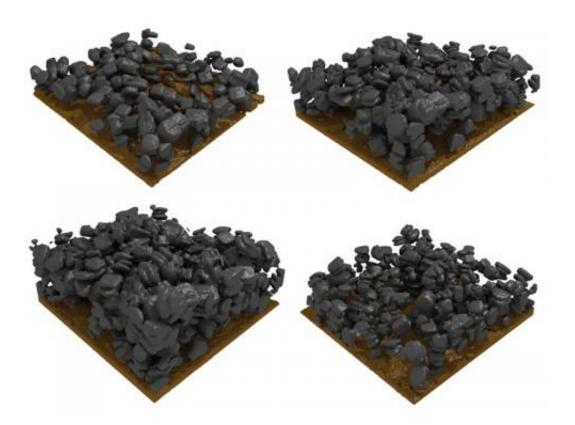
Particles of a tin oxide electrode experiencing structural changes during charging (images no 1-3) and discharging (3-4). Credit: Martin Ebner, Laboratory for Nanoelectronics, ETH Zurich
