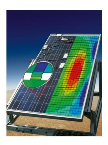
Sensors measure the elongations that arise in solar modules. Their operating life can be calculated from this data. Credit: © Fraunhofer IWM
