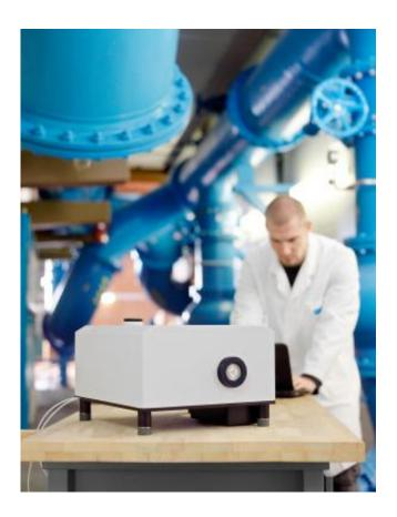
Little larger than a shoebox, the demonstrator was developed as part of the IRLSENS project. It is a quick and automated way to analyze water samples at the waterworks itself. Credit: © Martin Wagenhan / Fraunhofer IAF
