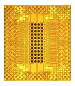
In the future novel optochips that combine lasers with electronics will dramatically reduce the size of technology devices (Holey Optochip image courtesy of IBM).
